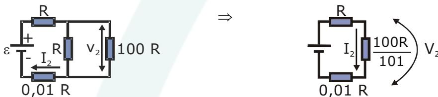
$$V_2 = \frac{100R}{101} \cdot I_2 \Rightarrow R_2 = \frac{V_2}{I_2} \Rightarrow \boxed{R_2 = \frac{100R}{101}}$$
