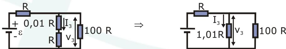
$$V_3 = 1,01R \cdot I_3 \Rightarrow R_3 = \frac{V_3}{I_3} \Rightarrow \boxed{R_3 = 1,01R}$$
