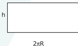
$$\begin{aligned} A &= 2\pi R h \\ A &= 2 \cdot 3 \cdot 1,70 \cdot 0,20 \\ A &= 2,04 \text{ m}^2 \\ A &= 2,0 \text{ m}^2 \end{aligned}$$
